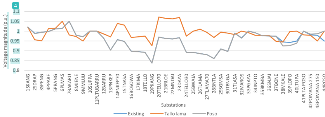
Fig. 7. Voltage profiles for initial condition, PV at Tallo Lama and PV at Poso
